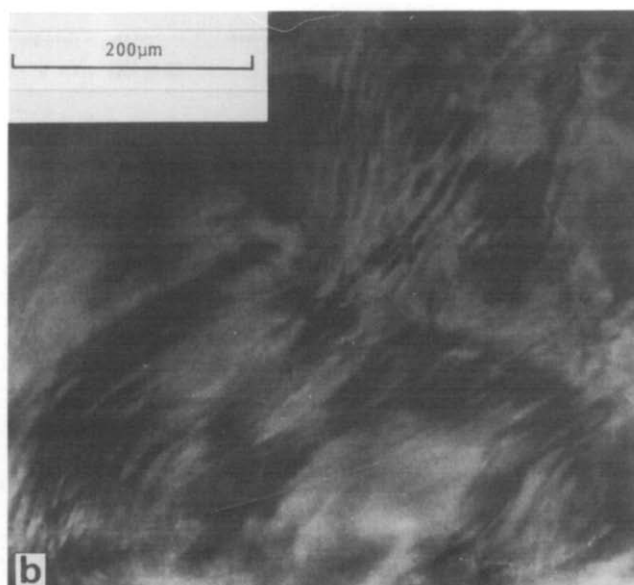
Figure 4 Optical micrographs under crossed polars of phase separation A: (a) top phase; (b) bottom phase
